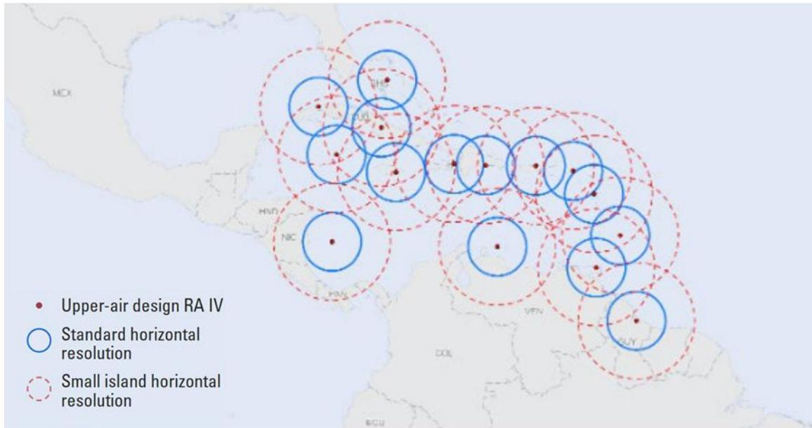
Figure 2. RA IV regional design of the upper-air GBON component with coverage of the Caribbean. The red dots indicate upper air stations, blue circles indicate the GBON standard horizontal resolution, while the red dashed circles refer to the GBON horizontal resolution for small islands.
